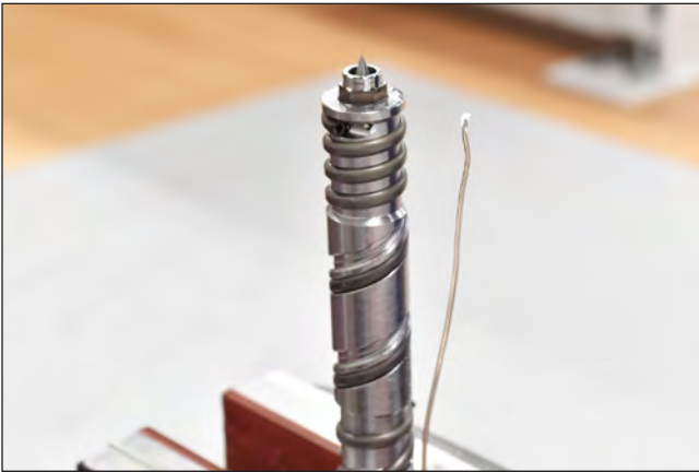
Picture 60: Coated tip of thermocouple
