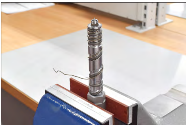
Picture 57: Disassemble the thermocouple
