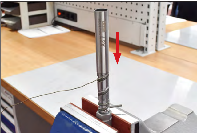
Picture 61: Installation of the new thermocouple
