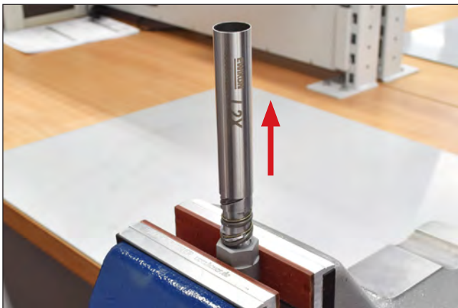
Picture 59: Pull off the protective tube
